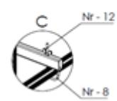
EN / Mount the struts under the platform: in platforms mounted at a height of 1.25 m.
